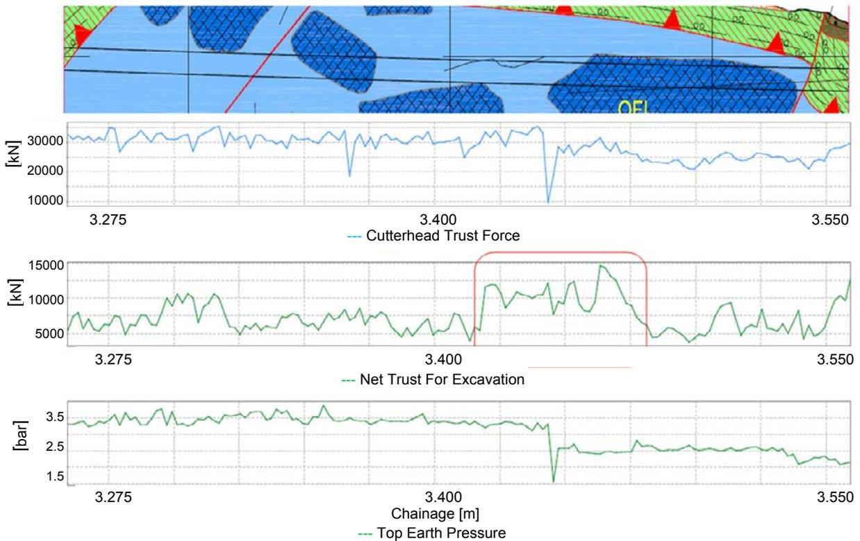
**Figure 5. Variability of the “Net Thrust for Excavation”**
