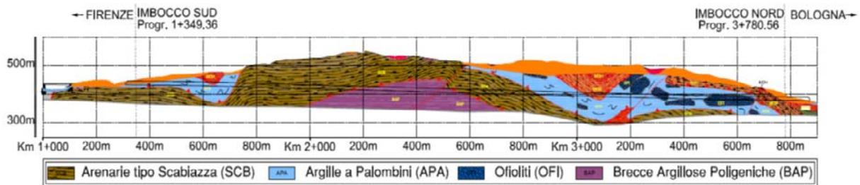
**Figure 1. Geological section of the Sparvo tunnel**
